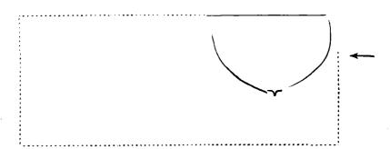
The straight side rests on a cliff and is practically unassailable. The only point from which attack can be anticipated is that shown by the arrow, as the ground on this side commands the interior of the work.
